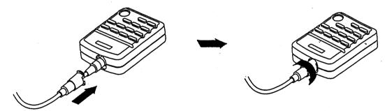
Connect the other end of the cable to the 8P connector on the front sub-panel of the main unit.
